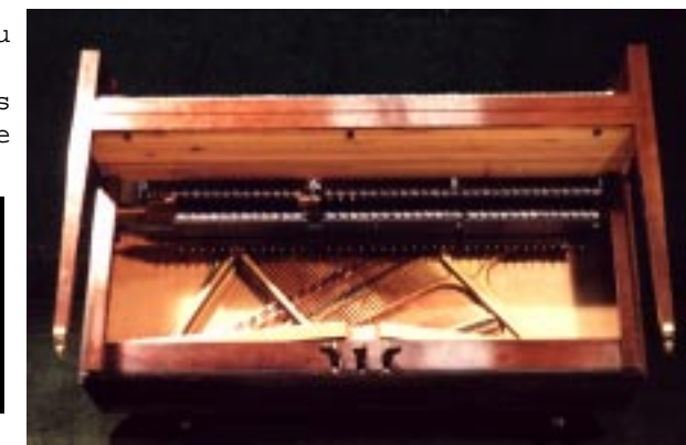
ST kit being installed Note ease of stack and roll frame placement and that the drums and tambourine fit without any modification of the cabinet!
