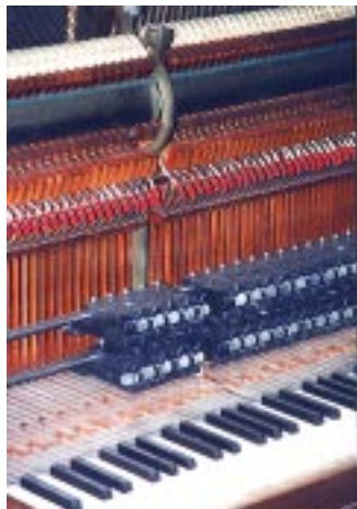
Pneumatic stack shown here installed in an upright piano.
